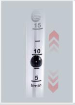
• Measure the gas flow (I/min) at the end of the torch by looking at the black ball.
